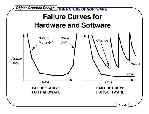
Hardware tends to have a wear-in time during which it has a higher probability of failure. This is generally referred to as *infant mortality*. Once the initial period is passed, hardware tends to operate without failure until components age enough to cause breakdown.
